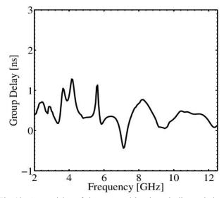
Fig. 12. Group delay of the proposed band-notch diamond shape UWB antenna
