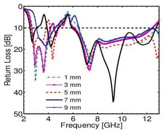
Fig. 8. Effect of the width  $W_s$  of the L-shaped slit on the simulated return loss of the dual band-notch UWB antenna; other parameters are the same as listed in Table 1
