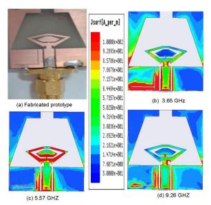
Fig. 6. Dual band-notched Diamond Shaped Monopole UWB antenna (a) Fabricated photograph (b) Current distribution at 3.65 GHz, (c) Current distribution at 5.57 GHz (d) Current distribution at 9.26 GHz.
