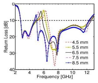
Fig. 5. Effect of the inner width  $W_{p3}$  of the C-shaped slot on the simulated return loss of the single band-notch UWB antenna; other parameters are the same as listed in Table 1
