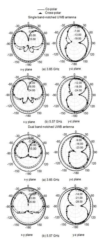
Fig. 10. Radiation pattern for various resonance frequency for the proposed UWB microstrip antenna with single and dual band-notched characteristics — Measured - - - Simulated at (a) 3.65 GHz (b) 5.57 GHz.
