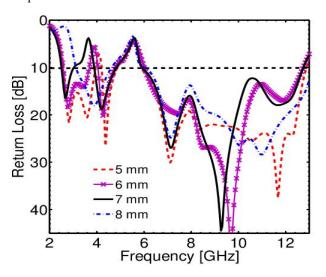
Fig. 7. Effect of the length  $L_s$  of the L-shaped slit on the simulated return loss of the dual band-notch UWB antenna; other parameters are the same as listed in Table 1
