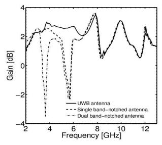
Fig. 11. Measured gain of the proposed diamond shaped UWB antenna, single band-notched diamond shape UWB antenna and dual band-notch diamond shape UWB antenna
