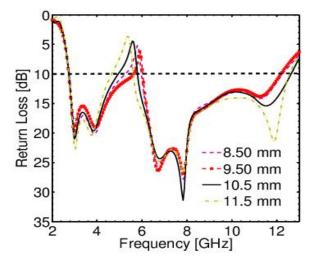
Fig. 4. Effect of the outer width  $W_{P2}$  of the C-shaped slit on the simulated return loss of the single band-notch UWB antenna; other parameters are the same as listed in Table 1
