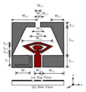
Fig. 1. Schematic configuration of the proposed dual band-notched diamond shaped UWB monopole antenna
