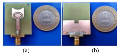
Fig.2. Photograph of the manufactured proposed antenna: (a) Top view (b) Bottom view
